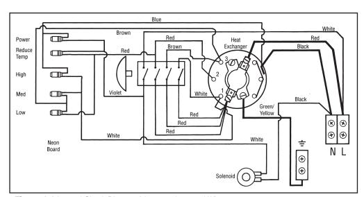
Figure 1.1 Internal Circuit Diagram (showers above 8.5kW)
