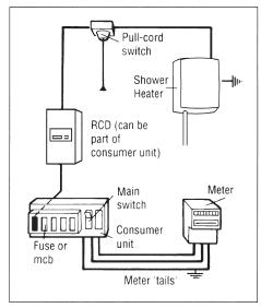
Figure 3.3 Schematic diagram of straightforward installation circuit
