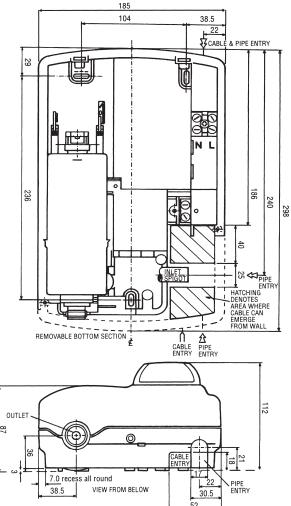
Figure 4.8 Backplate dimensions (in mm)
