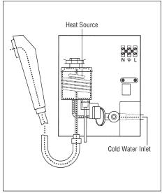
**Figure 1.17** Showing how the water is heated as it passes through.
