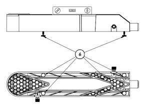
Put the shower tray over the Megaflo Horizontal SHRU and align it. Remove the tray for implementing the next steps.
