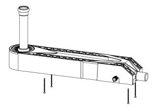
Make sure that the unit is installed horizontally. The internal bore of the Megaflo Horizontal SHRU already has a slope of 2% to ensure the correct flow of waste water from the shower.
