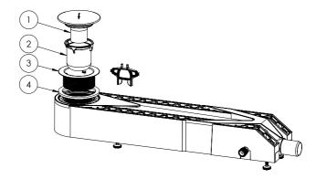
Using a spirit level and 4 adjustable feet (6) adjust the unit's height and position it horizontally in its final location. The internal bore of the Megaflo Horizontal SHRU already has a slope of 2% to ensure the correct flow of waste water from the shower.
