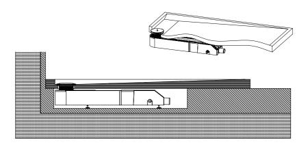
4.2.2 Installation under the slab / under the shower tray or bathtub
