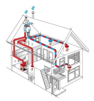
The central unit of the balanced ventilation system in your home is the HRU ECO 4 (heat recovery unit). This unit has two motors. One motor for air extraction and one for air supply. Air is extracted from the kitchen, bathrooms, en-suites, utility rooms and toilets and, if required, from a storage room. In larger properties more than one unit may have been installed.
