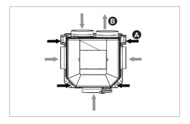
Using suitable screws in the mounting holes, mount the ventilation unit on a vertical or sloping wall, ceiling or floor with sufficient load-bearing capacity (> 200 kg/m²), preferably in a closed room. (A)
