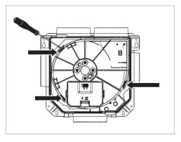
d) Remove the motor plate with the motor, impeller and circuit board enclosure.
