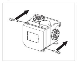
b) The capacity at high speed (H) and low speed (L) can be adjusted with the two potentiometers.
