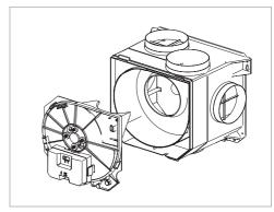
clean the fan impeller with a soft brush. Be careful to avoid dislodging any balancing clips on the fan impeller.
