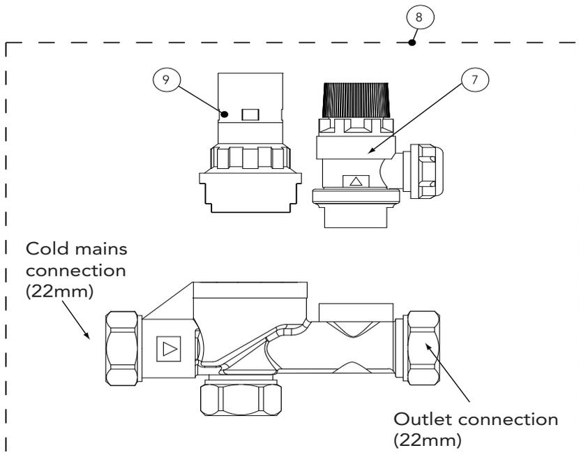
Figure 12: Exploded view of cold water combination valve
