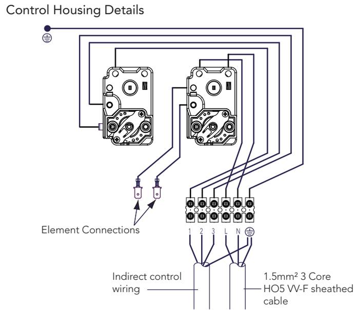
Figure 4: Indirect wiring schematic
