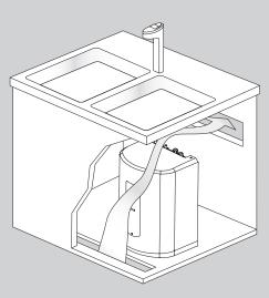
Air circulation must be provided so air can flow through the cupboard. Failure to do this may result in the Aquatap not performing correctly.
